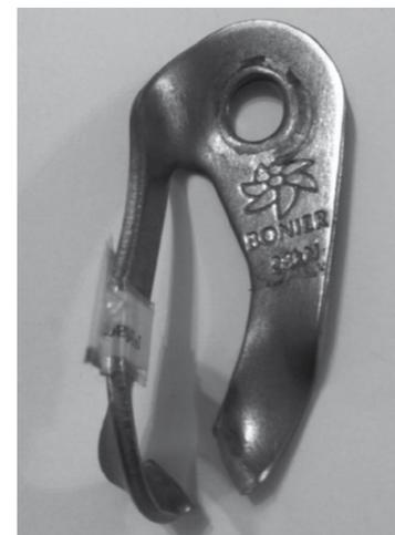
Chapeleta Bonier ensaiada, ruptura 30,87kN,
